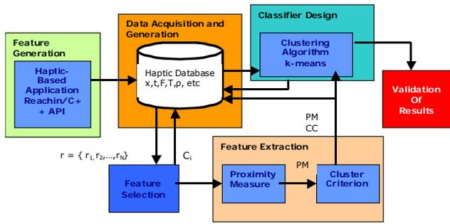
**Figure 2. The proposed dynamic haptic-based authentication system.**
