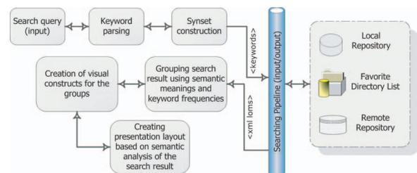
**Figure 1. Architecture illustrating the grouping and presentation style creation steps in the 3D car metaphor**
