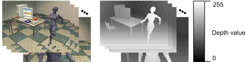
**Fig. 1.** Depth image-based representation with color and synchronized depth images
