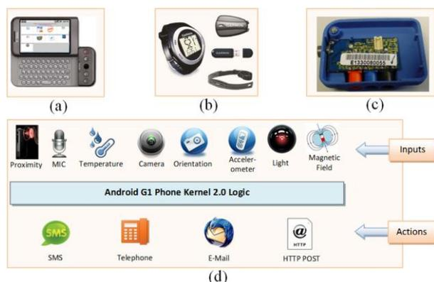
Fig. 6. Sensors and smart phone used to evaluate the framework (a) An HTC dream running Android 2.0, (b) Garmin Forerunner heart beat sensor, (c) SHIMMER ECG kit, and (d) Built-in sensors and communication channels comes with the HTC smart phone.
