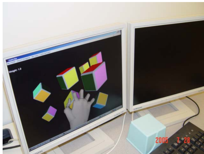
Fig. 3 Arranging cubes in an arbitrary way to test the grip of the user
